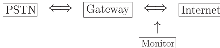
FIG 1. Global Crossing location in Newark New Jersey. A monitor with an Endace card collected packet headers and timestamps of both directions of calls using a link between an IP-PSTN gateway and an IP network edge router.
